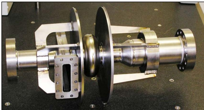
Figure 3: Third Harmonic Injector Corrector Cavity.
