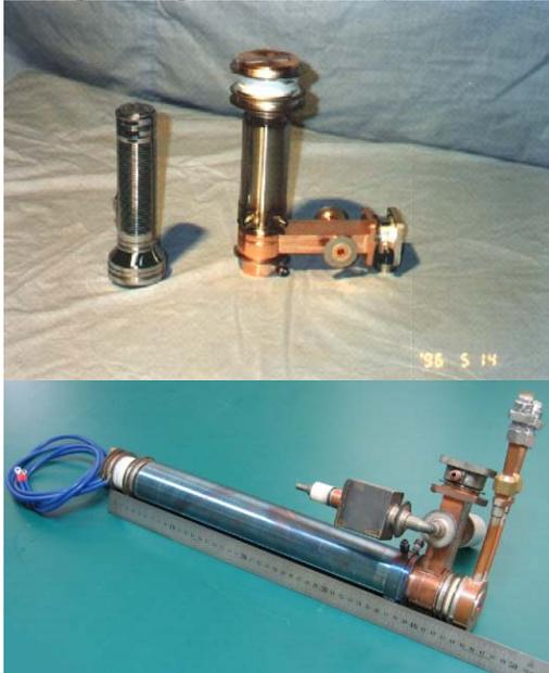
Figure 2: X-band accelerating tubes, 2.5MeV (upper) and 6MeV (lower).
