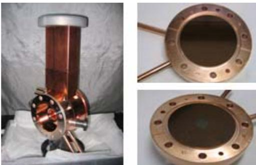
Figure 1: Pictures of the photocathode rf gun, left-up is copper and left-down is magnesium cathode.
