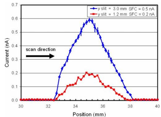
Figure 3: Results of BH FC scans of the Pelletron 10 MeV proton beam.
