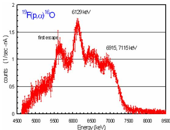
Figure 4: Background subtracted NaI(Tl) spectrum of gammas from LiF irradiation by 10 MeV protons.
