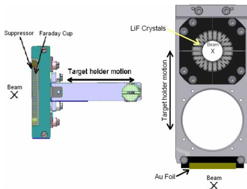
Figure 1: Left – The special Faraday Cup for the direct charge measurements. Right – Target holder for the nuclear techniques. Possible beam positions (entering the page) and targets motions are shown.
