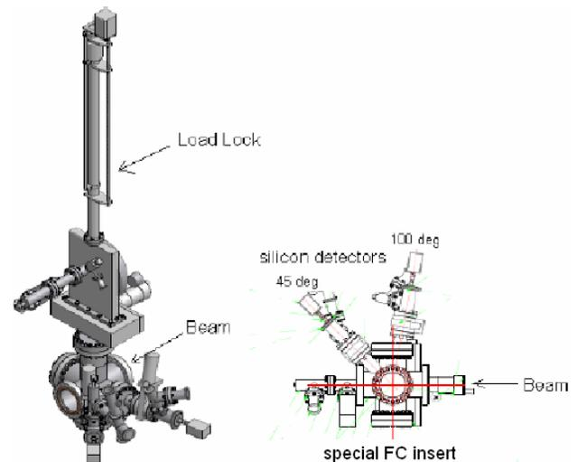
Figure 2: Left – 3D view of the BH monitor vacuum chamber. Right – Bottom view of the BH monitor.
