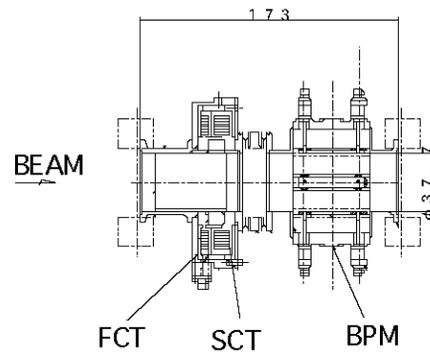
Figure 7: Mechanical design of MEBT monitor (type 2). In this figure beam runs from left (FCT) to right (BPM). Monitors are welded with each other.
