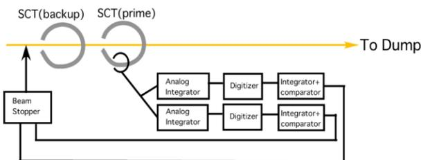
Figure 3: Schematics of the interlock system for total number of accelerated particles. SCT provides elementary information for the system.
