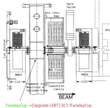
Figure 1: Schematic view of LEBT [1]. Green and red letters show existing and upgraded monitors, respectively.
