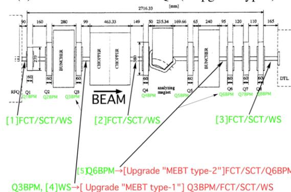
Figure 2: Schematic view of monitor location for MEBT [1]. Green and red letters show existing and upgraded monitors, respectively.
