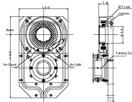
Figure 4: SCT monitor in LEBT. A faraday cup detector is also mounted on the same detector head. Depending on the functionality, either the SCT or the Faraday cup is on the beam line (mechanically moved by a stepping motor).
