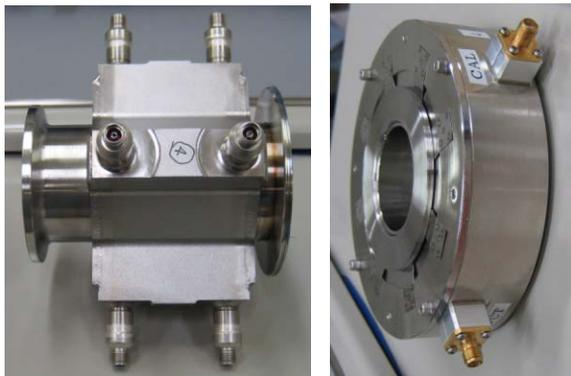
Figure 6: BPM (left) and FCT+SCT(right), before weld.
