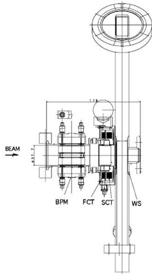
Figure 5: Mechanical design of MEBT monitor (type1). In this figure beam runs from left (BPM) to right (WS). Monitors are welded with each other.
