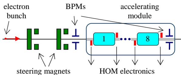
Figure 3: Calibration setup.
