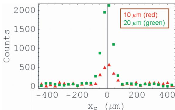
Figure 4: The signal strength for BFW with diameter of  $10 \mu\text{m}$  (red) and  $20 \mu\text{m}$  (green).
