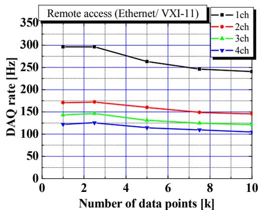
Figure 5: Result of the data acquisition speed by a remote access.
