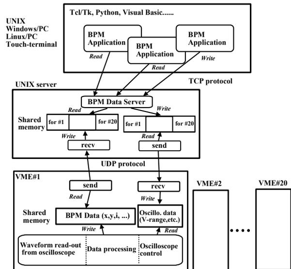
Figure 3: Block diagram of the control software and data flow.
