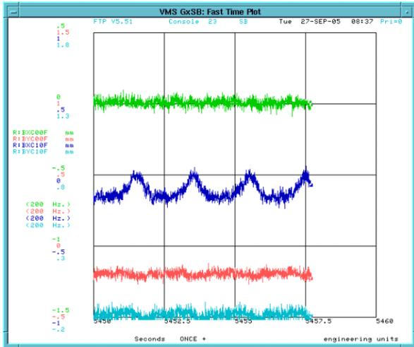
Figure 4: Beam positions with damper off.
