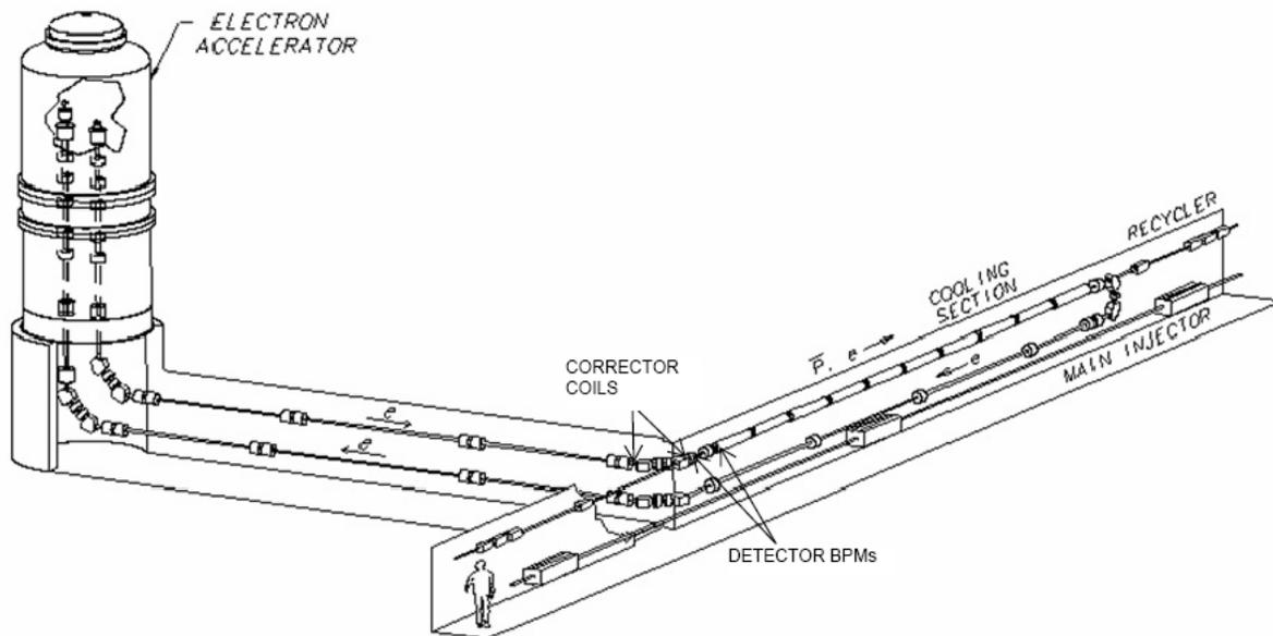
Figure 1: Location of damping system components.
