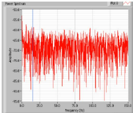
Figure 7: Noise spectrum with damper on.
