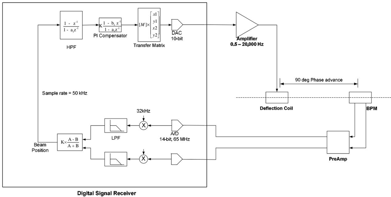
Figure 2: Damper system hardware.
