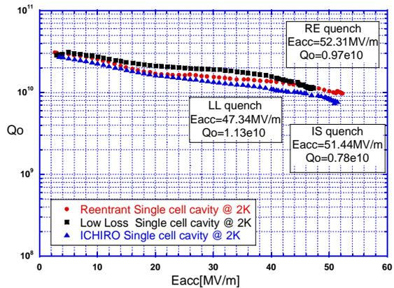
Figure 2: The best result of each cavity shape.
