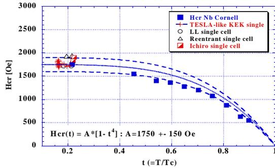
Figure 3: The experimental RF critical field.
