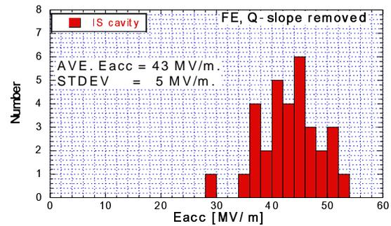
Figure 6: Histogram of the gradient in the tests.
