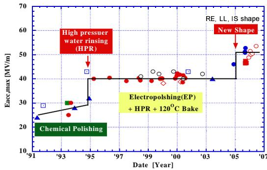
Figure 4: The breakthrough to 50MV/m.
