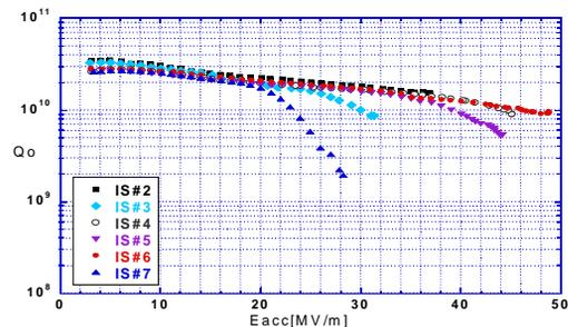
Figure 5: The first trial results for six IS cavities.
