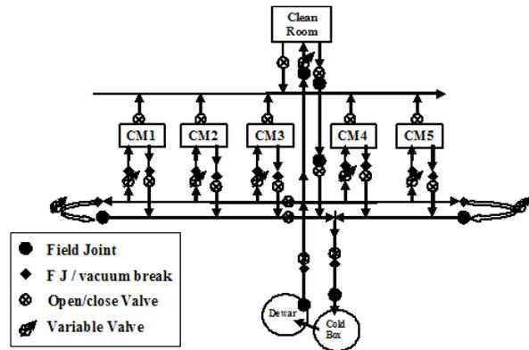
Figure 3: Schematic of the ISAC-II LHe distribution system.
