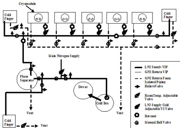
Figure 5: Schematic of the ISAC-II Nitrogen distribution system.
