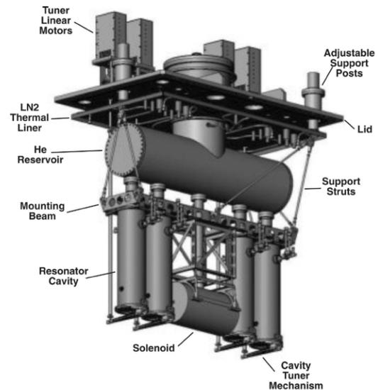
Figure 2: Cryomodule top plate assembly.
