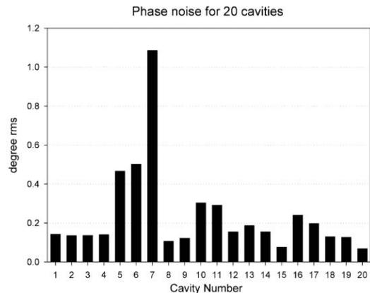
Figure 6: Phase noise measured for each cavity.
