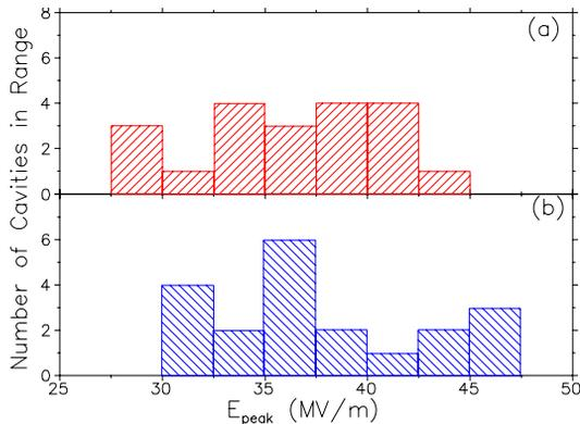
Figure 5: Distribution of cavity peak surface field for both the *in situ* cavities (a) and the single cavity tests (b).
