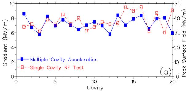
Figure 4: Average cavity gradients for the three  $A/q$  values and for 7 W cavity power. Results are inferred from the step energy gain per cavity during acceleration. Also shown are gradients from initial single cavity characterizations.
