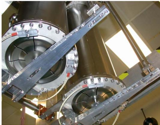
Figure 2: Photo of tuning plate and tuning lever mechanism.
