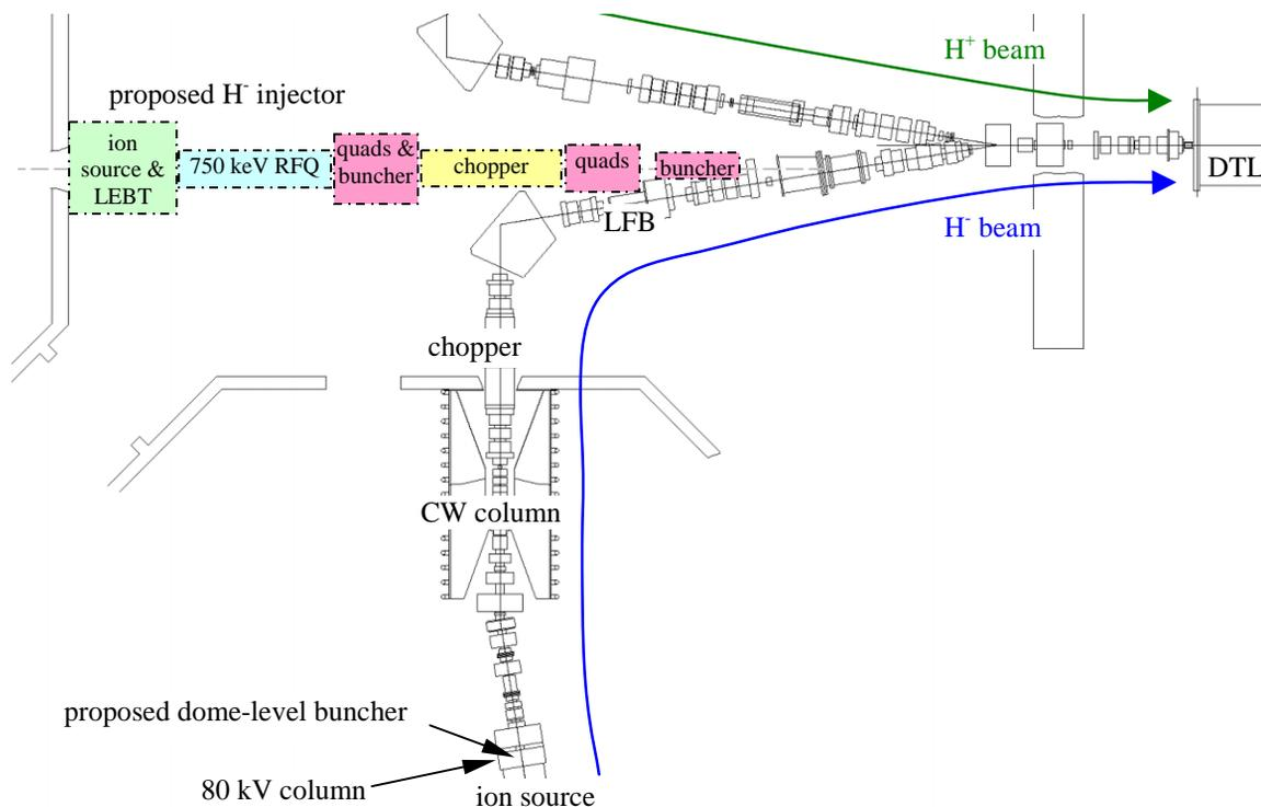
Figure 1: Partial top view of LANSCE injectors with proposed RFQ-based injector and dome level buncher shown schematically.
