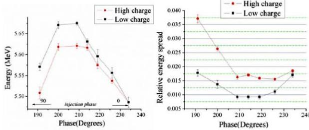
Figure 3. Beam energy and energy spread as functions of the launching phase.
