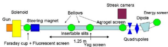
Figure 1: Block diagram for first phase of SPARC photoinjector commissioning.
