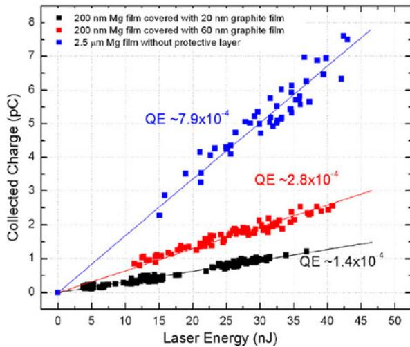
Figure 6: Emission curves of different Mg samples deposited by PLD on Cu substrates, after the laser cleaning of the protective or contaminated layers.
