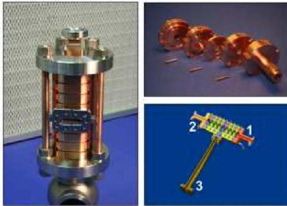
Figure 7: Copper prototype of the structure.
