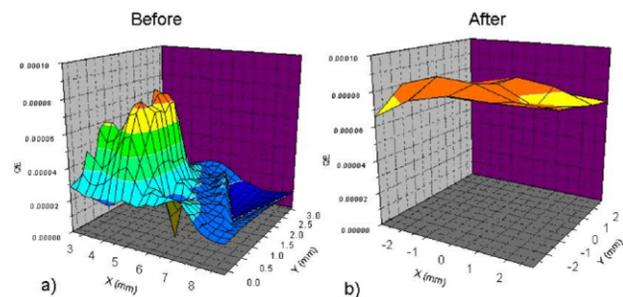
Figure 2: Quantum efficiency map before (a) and after (b) the laser cleaning procedure.
