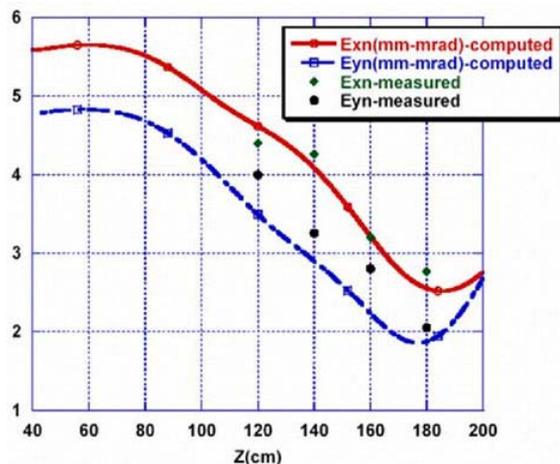
Figure 4. Measured emittance along  $z$  compared with Parmela simulations.
