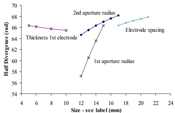
Figure 2: Beam divergence as a function of the parameters of a diode post-acceleration system.
