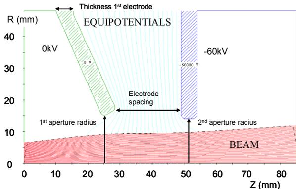
Figure 1: Simulation of post-acceleration system.
