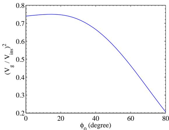
Figure 5: The ratio of the cathode-cell impedances defined by Eq. (2) and Eq. (1) as a function of launch phase.
