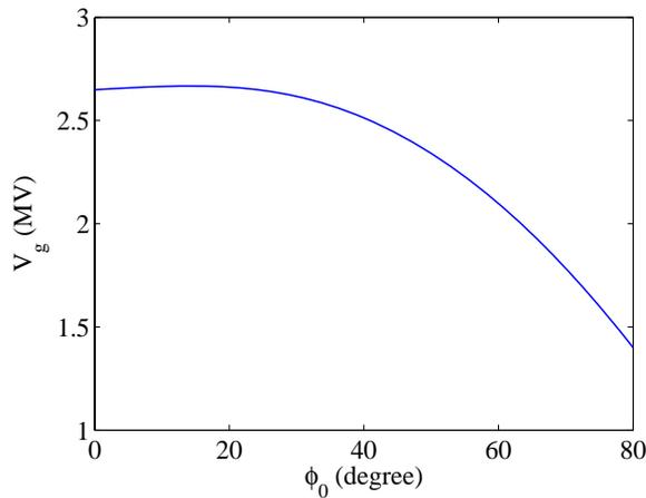
Figure 4: Beam voltage gain in the cathode cell as a function of launch phase.
