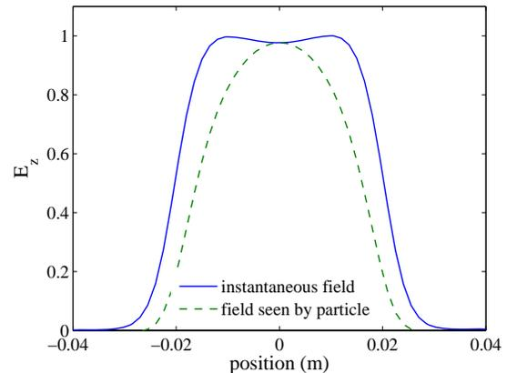
Figure 3: The instantaneous longitudinal electric field and the field seen by the particle inside the full cell.
