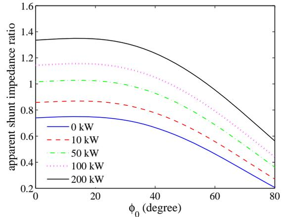
Figure 6: The apparent shunt impedance ratio at different full-cell residual power levels.
