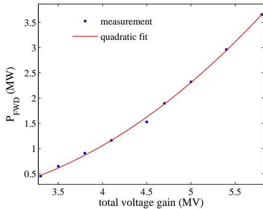
Figure 2: The forward power of the first full cell versus the total voltage gain from the cathode cell and the first full cell.
