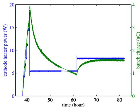
Figure 2: Bunch charge (green) versus time as the cathode heater power (blue) is varied.
