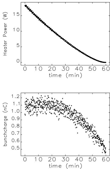
Figure 1: (top) Cathode heater power is varied gradually over time; (bottom) the corresponding bunch charge delivered as a function of time.
