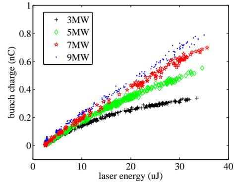
Figure 3: Bunch charge versus UV laser beam energy at different klystron output power.
