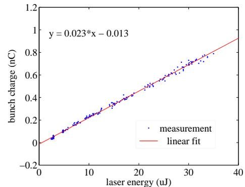
Figure 4: A linear fit of bunch charge versus laser beam energy as measured by the energy meter in the laser room.
