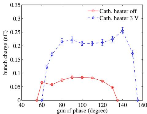
Figure 5: Measured bunch charge versus rf phase at different cathode heater voltages.
