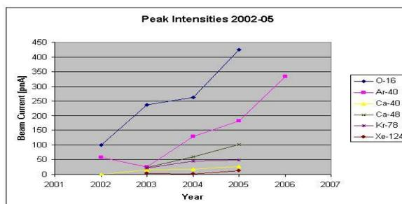
Figure 6: Peak current extracted (at ~140 MeV/u) by year from 2002 to mid-2006. Beams are O, Ar, Ca, Kr, and Xe. A peak beam power of 2 kW was achieved with  $^{40}\text{Ar}$  in January 2006 with more sustained values of ~1.5 kW.
