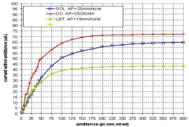
Figure 3: Measured  $^{40}\text{Ar}^{7+}$  current contained within a defined emittance with the DDS (top line), solenoid (middle), and LBT (bottom). Switching the octupole element of the DDS on results in ~10% gain in beam current compared to off.
