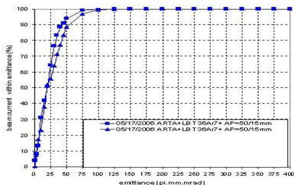
Figure 4: Percentage of total beam vs. emittance is plotted for  $^{36}\text{Ar}^{+7}$  in the best case from Table 1.
