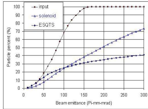
Figure 2: Percentage of total beam vs. beam emittance from a simulated output of ARTEMIS. The solenoid transmits more beam at higher emittance, but less at the low emittance required for K500 injection.
