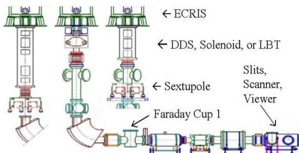
Figure 1: Injection beam line layout showing some element arrangements tested. The distance from ECR to analysis magnet is about 2.2 m.
