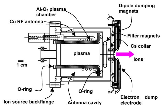
Figure 1: Schematic diagram of the prototype SNS external antenna ion source.
