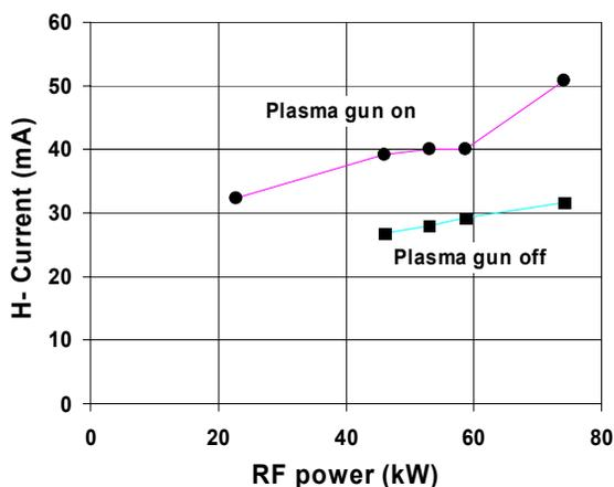
Figure 5: Extracted  $H^-$  beam current with and without the plasma gun activated.
