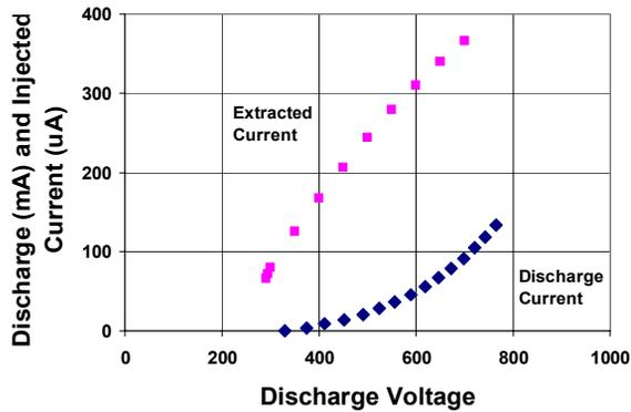
Figure 4: Discharge (anode-cathode) current and extracted current at  $H_2$  flow was 50 SCCM.
