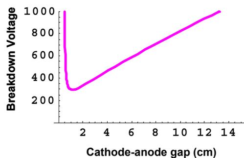
Figure 3: Paschen voltage breakdown curve for a simple glow-discharge calculated for pressures of 1 Torr of H<sub>2</sub>.
