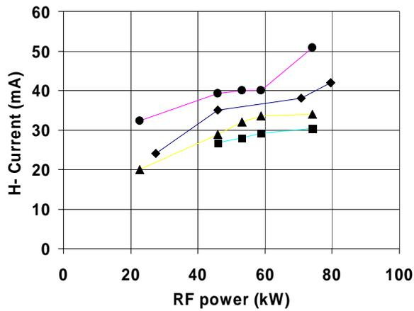
Figure 1: Extracted  $H^-$  beam current versus applied RF power: squares – air cooling, plasma gun deactivated; circles – air cooling, plasma gun activated; triangles – liquid cooling, plasma gun activated; diamonds – air cooling, plasma gun activated, Faraday shield inserted (Fig. 2).
