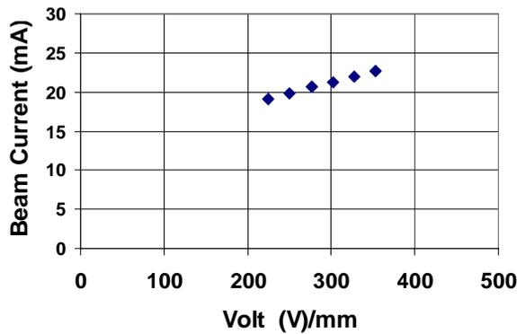
Figure 4: Beam current plotted against electric field strength at outlet aperture adjusted by varying the extraction potential (see text).
