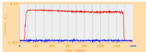
Figure 3: Example  $H^-$  pulse (33 mA, 1.2 ms in length) extracted from the prototype ion source.
