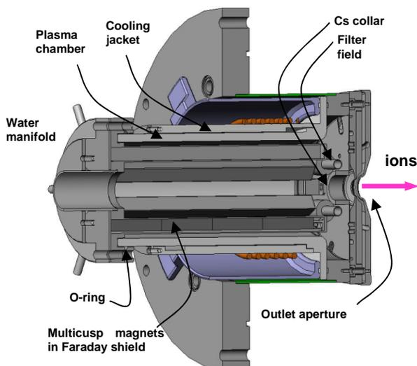
Figure 5: The high-power external antenna source.
