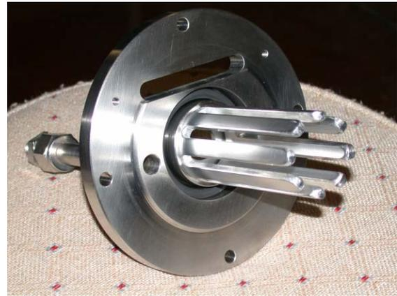
Figure 2: Metallic Faraday shield and backflange inserted into the ceramic plasma chamber of the prototype ion source.
