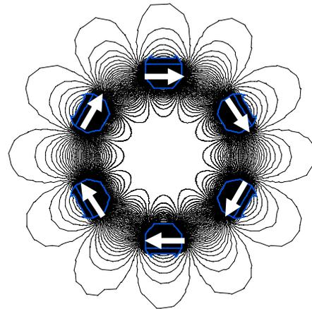
Figure 6: Magnetic field pattern which results from the multicusp configuration used in the high-power source.
