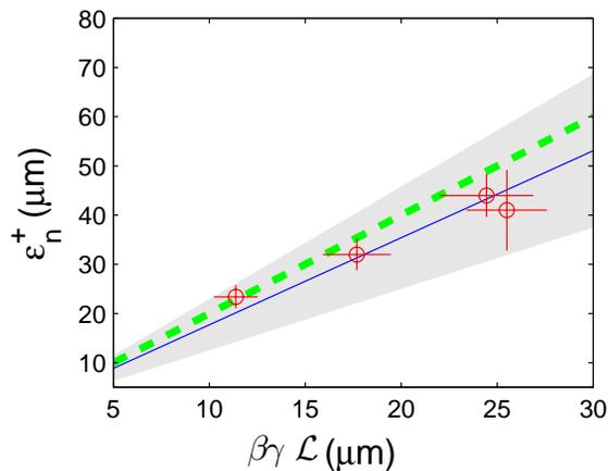
Figure 2: Larger one of the flat beam emittances ( $\varepsilon_n^+$ ) versus  $\beta\gamma L$ . A linear regression (solid line) of the experimental data (circle) is compared with the theoretical dependence (dashed line). The shaded area represents the 95% confidence bounds associated with the linear regression.
