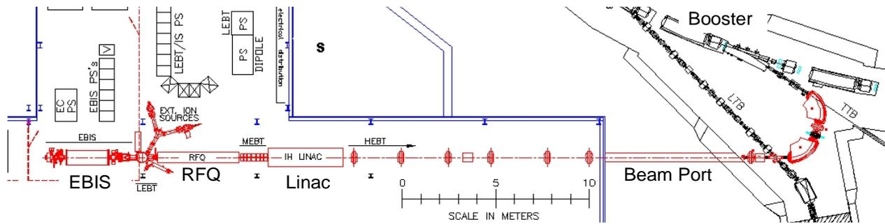
Fig. 1: Layout of the EBIS Preinjector
