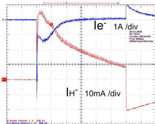
Figure 2: Oscillogram of the longest and highest H<sup>+</sup> beam puls extracted from any volume source.
