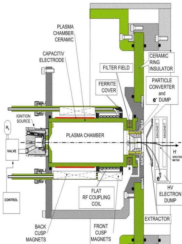
Figure 1: The NEW HERA RF-Driven Multi cusp H<sup>-</sup> Ion Source.
