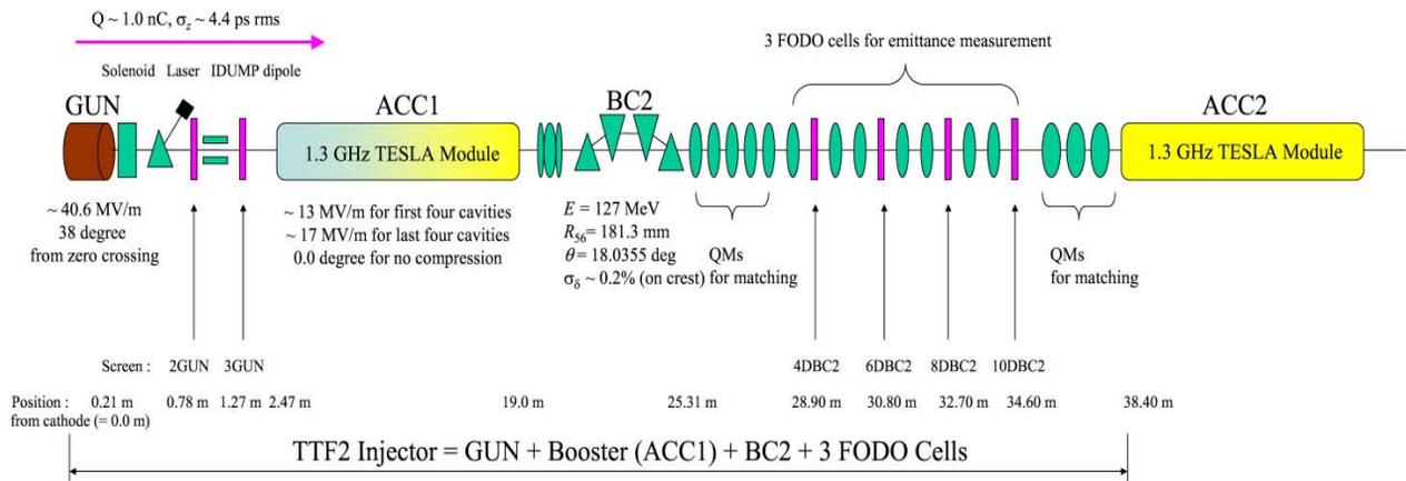
Figure 1: Layout of TTF2 RF photoinjector.
