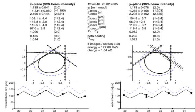
Figure 3: Measured transverse emittance with 90% core intensity on February 23rd, 2005.
