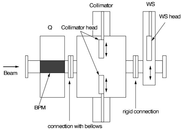
Figure 2: Monitor layout around a collimator.
