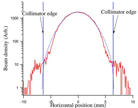
Figure 3: Typical beam profile at a collimator location (simulation). Top: linear, bottom: logarithmic. The dotted line shows the Gaussian fit.
