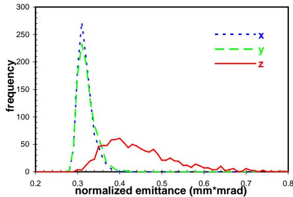
Figure 2: Output beam emittances with standard errors.
