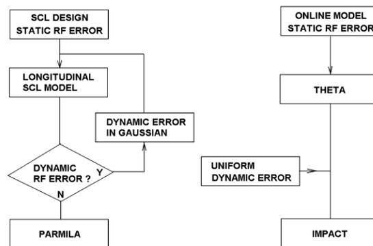
Figure 1: SC linac models built for simulation study.
