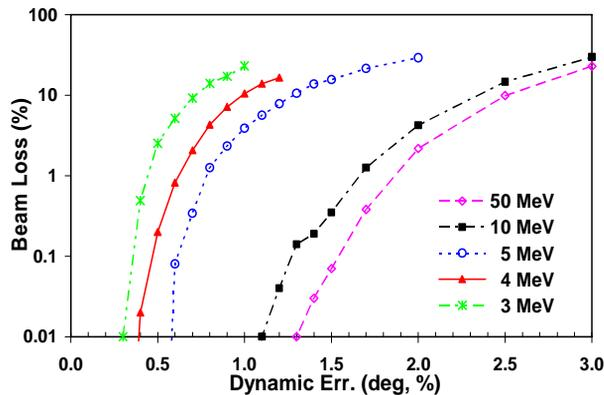
Figure 6: Beam loss in various energy tails depends on dynamic RF errors of the superconducting linac.
