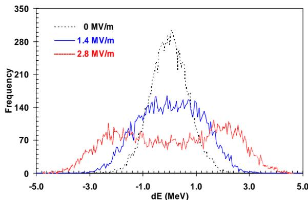
Figure 7: Beam energy distributions with the last cavity as an energy spreader, for dynamic RF errors of  $\pm 0.3^\circ$  and  $\pm 0.3\%$  in the superconducting linac.
