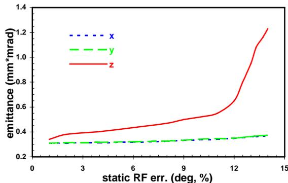
Figure 3: Beam emittances versus static RF errors in SCL high beta section.
