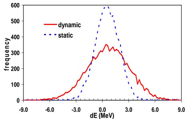
Figure 5: Beam energy jitters for dynamic RF errors and for static RF errors, both of  $\pm 1^\circ$  and  $\pm 1\%$ .
