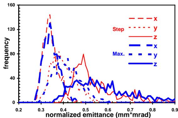
Figure 4: Beam emittances with the maximum acceptable static RF errors:  $3^\circ$  and 5% (Max.) and with the high beta cavity errors:  $10^\circ$  and 10% (Step).
