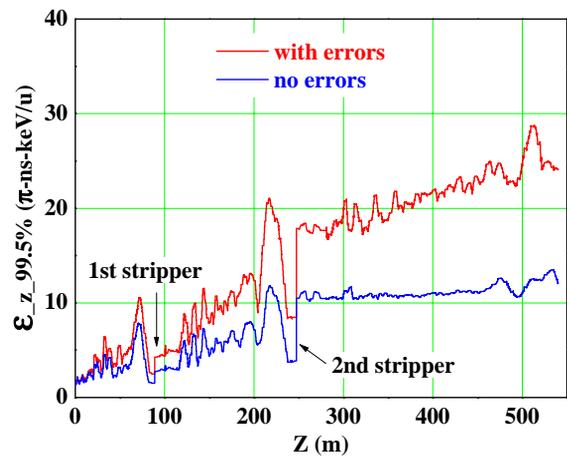
Figure 6: Longitudinal emittance with and without errors along the superconducting linac.
