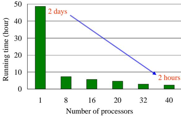
Figure 2: Running time versus number of processors for 1.6-million-particle tracking throughout the SC linac on the high performance computers at MSU.
