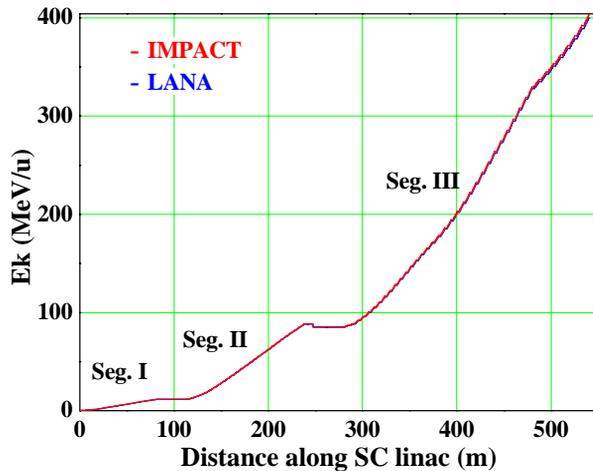
Figure 3: Energy gain along the superconducting linac with IMPACT and LANA code.
