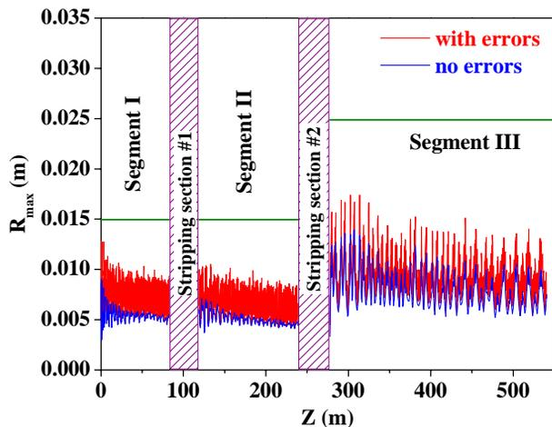
Figure 5: Maximum beam envelope along the superconducting linac with and without errors. Minimum beam apertures in each segment are shown as well.
