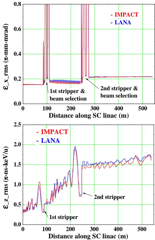
Figure 4: Horizontal (top) and longitudinal (bottom) rms emittances along the superconducting linac with IMPACT and LANA codes. Vertical emittance is not shown but similar to horizontal one.
