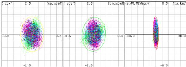
Figure 3: Phase space portraits of  $^{238}\text{U}^{71-75+}$  at the charge stripping foil 2 ( $f_{rf}=322$  MHz).
