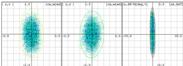
Figure 4: Phase space portraits of  $^{238}\text{U}^{87-89+}$  after the charge stripping foil 2 ( $f_{rf}=322$  MHz).
