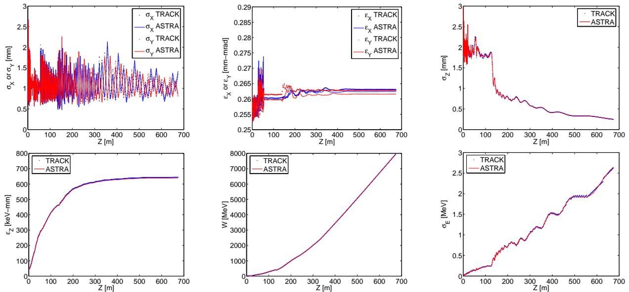
Figure 2: TRACK and ASTRA simulations of the High-Intensity Proton Source for Zero Current, from the RFQ exit to the last accelerating cavity. From top left to bottom right : transverse RMS size, transverse RMS normalized emittance, RMS bunch length, longitudinal RMS normalized emittance, kinetic energy and RMS energy spread.
