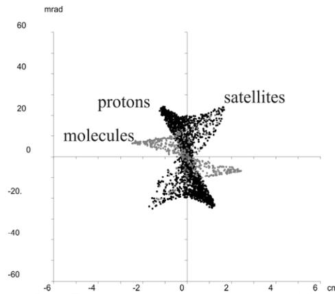
Figure 5: Emittance pattern with "Satellites",  $B1 = 129 \text{ mT}$ ,  $B2 = 114 \text{ mT}$ .
