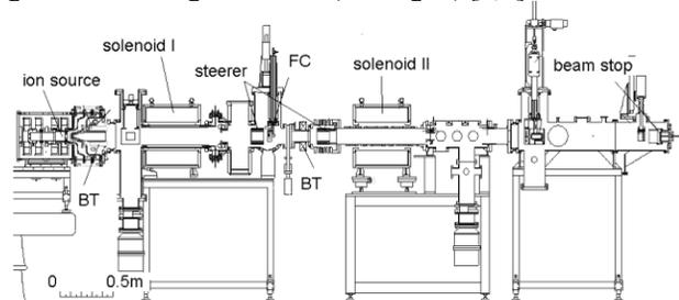
Figure 1: Schematic drawing of the SILHI-LEBT [3].
