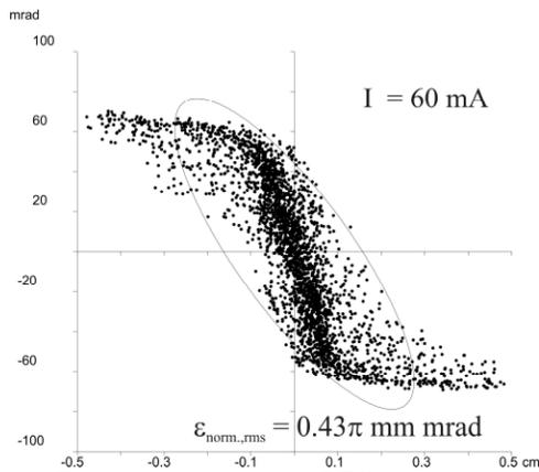
Figure 4: Emittance pattern for RFQ injection according to the beam plasma model.
