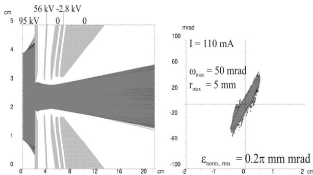
Figure 2: Extraction system, trajectory plot (left), emittance pattern (right).
