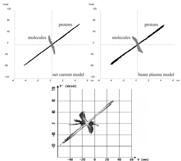
Figure 3: Calculated and measured phase space distributions: net current model (left), beam plasma model (right), parallel beam after solenoid 1 (B1 = 129 mT) and subsequent focussing after solenoid 2 (B2 = 215 mT); measurement (lower).
