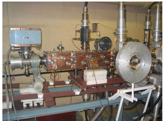
Figure 1: 1 MeV 433 MHz deuteron linac on the laboratory stand.
