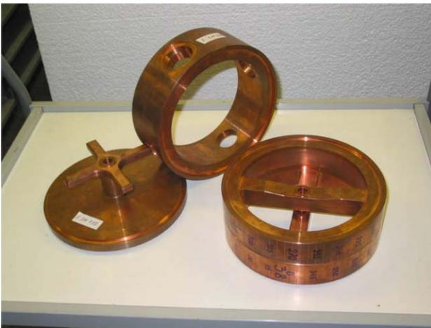
Figure 3: Elements of 433 MHz structure with alternate phase focusing.
