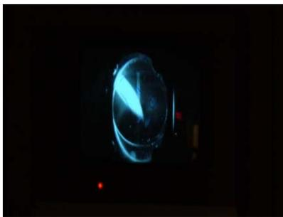
Figure 9: First electrons from the 350 keV photoinjector, imaged onto a YAG screen.
