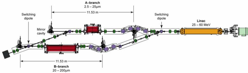
Figure 3: Schematic layout of the 4GLS IR-FEL. Two undulators give wavelength tuneability over 2.5 to 200 um.
