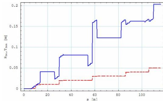
Figure 6: First (red/dashed) and second (blue/solid) order longitudinal dispersion values in the HACL insertion device arcs. An  $R_{56}$  of 1 cm/cell provided by each triple-bend achromat cell [2] gives progressive compression of the 77 pC bunches. The  $R_{56}$  is tuneable to zero to allow other modes of operation.
