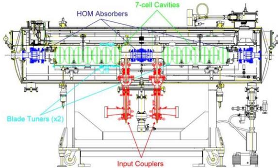
Figure 4: Prototype cryomodule incorporating two 7-cell modified TESLA-type cavities.
