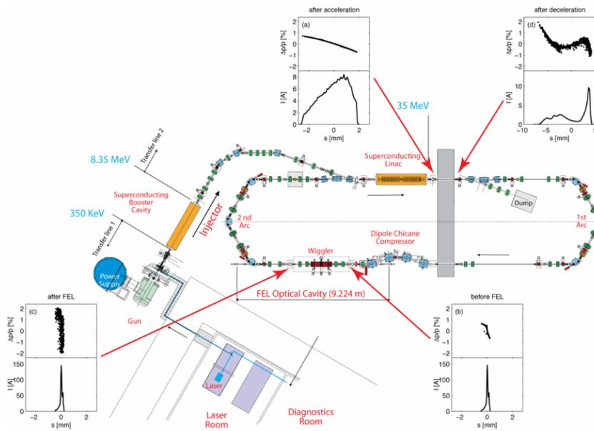
Figure 8: Layout of ERLP, showing typical beam distributions obtained from start-to-end simulation which include the effect of the IR-FEL lasing process [4]. The existing building shield wall is shown in grey.
