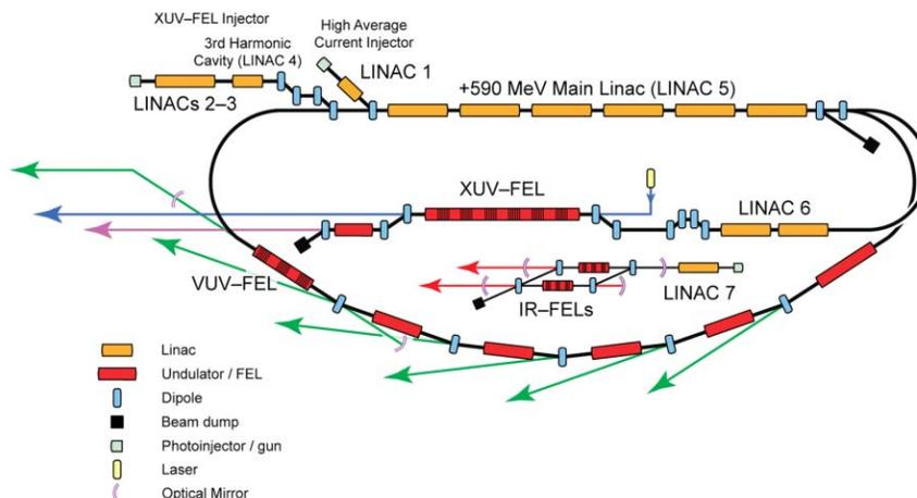
Figure 2: The conceptual layout of 4GLS.
