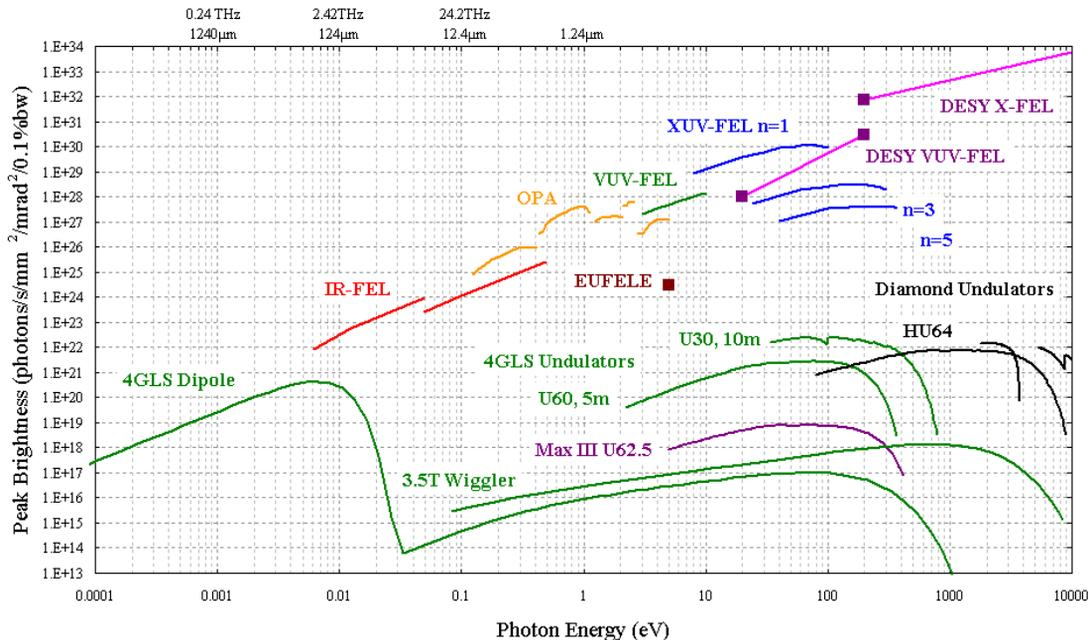
Figure 1: Peak brightness values for the 4GLS FELs, undulators, wiggler, OPA and dipoles compared with EUFELE, X-FEL, DIAMOND and Max III undulators.
