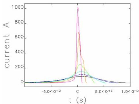
Figure 7: Progressive compression from HACL Straights 1 to 6 gives bunch lengths from  $\sim 900$  fs (black) down to  $\sim 100$  fs (pink).
