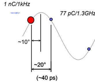
Figure 5: Principle of opposing-phase compression proposed for 4GLS.
