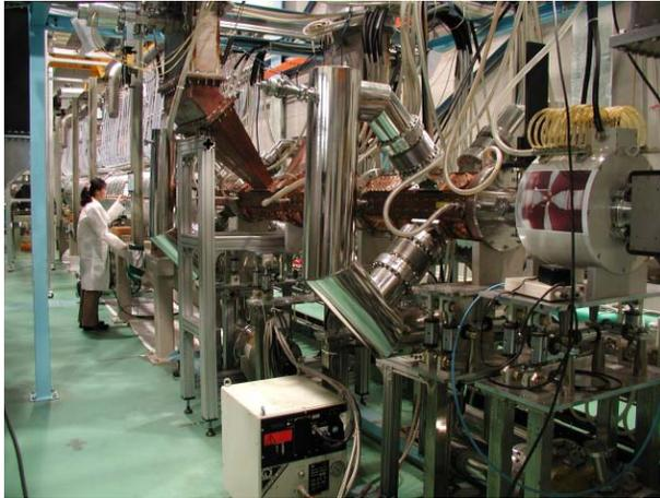
Figure 2: 20 MeV proton accelerator installed at KAERI test stand.
