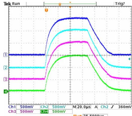
Figure 6: Field profiles in four tanks of DTL1 (blue : tank 1, jade : tank2, pink : tank3, green : tank4).
