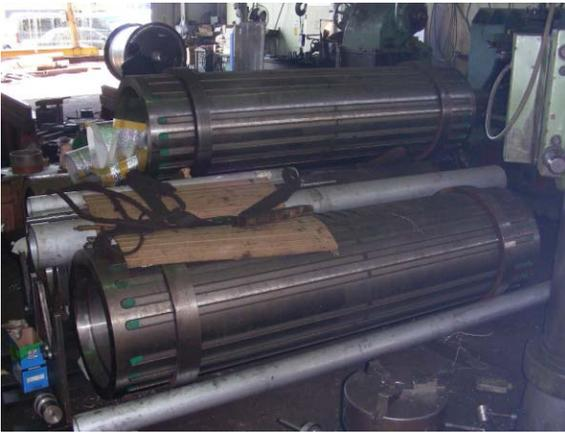
Figure 8: Machined DTL2 tanks.
