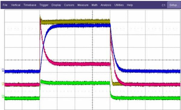
Figure 4: RF signals after high power rf conditioning (yellow : Forward, red : reverse, blue : cavity, green : klystron reverse).
