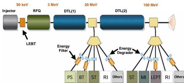
Figure 1: PEFP proton linac and user beam lines.
