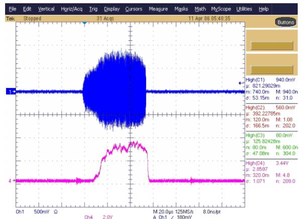
Figure 7: Beam signal of the 20 MeV DTL (CH1:  $\sim 1\text{mA}$  at RFQ exit, CH2:  $\sim 1\text{mA}$  at DTL exit).
