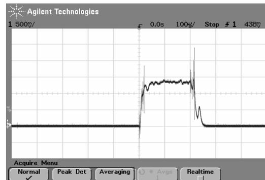
Figure 3: Beam signal at the LEBT exit (1mA/div., 200  $\mu$ s pulse).
