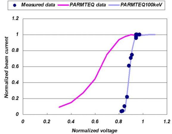
Figure 5: RFQ output current depending on RF field (Red line : total beam current, Blue line : accelerated beam current, Dot : measured beam current)
