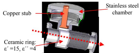
Figure 19: Beam line absorber for the European XFEL facility.
