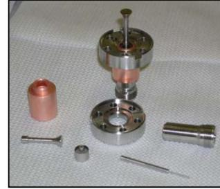
Figure 8: Parts of the feedthrough with improved heat conduction. *Courtesy of JLab.*
