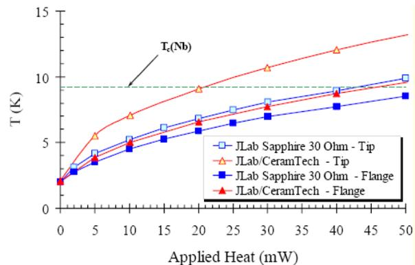
Figure 9: Thermal test results  $T$  vs. heat applied to the antenna tip. *Courtesy of JLab.*
