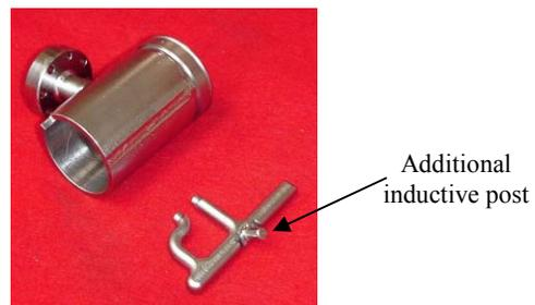
Figure 10: Parts of the HOM coupler with the hidden antenna.
