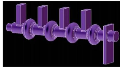
Figure 13: Weakly coupled 1.5 GHz cells with waveguide HOM couplers proposed in [9].
