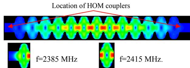
Figure 1: Example of mode trapping in a 13-cell cavity. End-cells and inner-cells have different frequencies for this resonant pattern.
