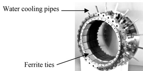
Figure 17: Ferrite beam line absorber used for CESR cavity.
