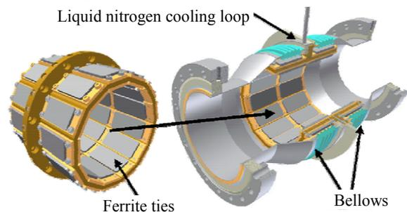
Figure 18: Ferrite beam line absorber as proposed at present for the ERL at Cornell.
