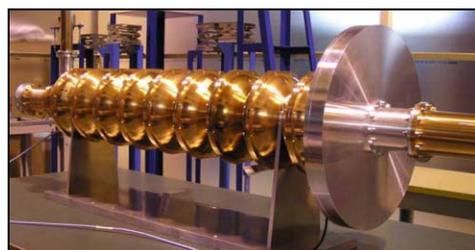
Figure 16: TESLA 9-cell structures with circular damper.
