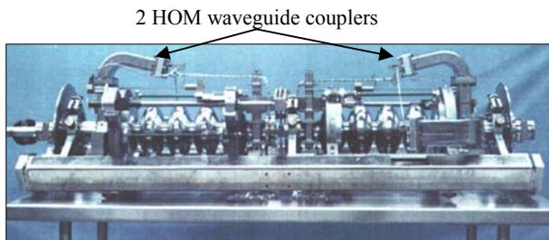
Figure 12: Pair of 5-cell 1.5 GHz CEBAF cavities with HOM waveguide couplers.
