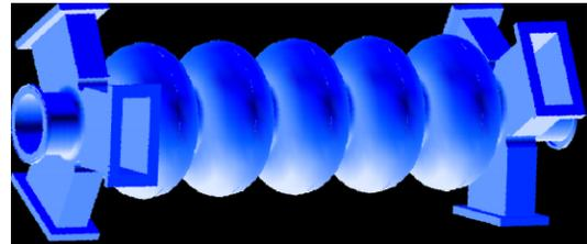
Figure 14: 750 MHz 5-cell structure with six waveguide HOM couplers discussed in [10].
