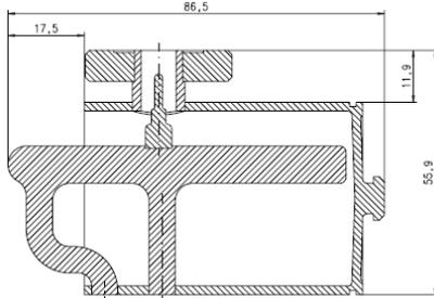
Figure 11: HOM coupler with direct connection between its inner conductor and the feedthrough.
