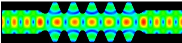
Figure 4: 5-cell 704 MHz structure for the electron cooling at RHIC.
