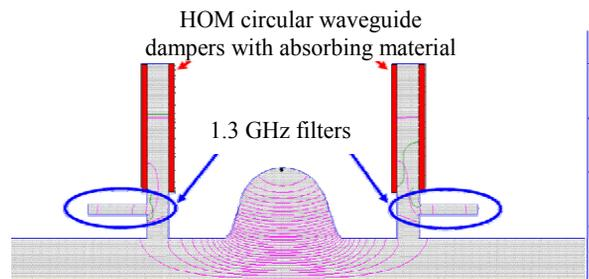
Figure 15: Two circular HOM dampers as modeled with single TESLA cell.
