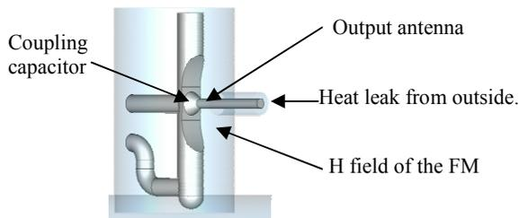
Figure 7: Heat sources in the coaxial HOM coupler.
