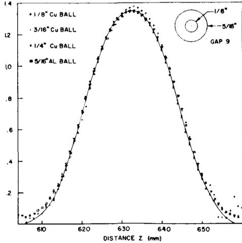
Fig. 5. Field distribution in gap 9 as measured with four different ball sizes.
