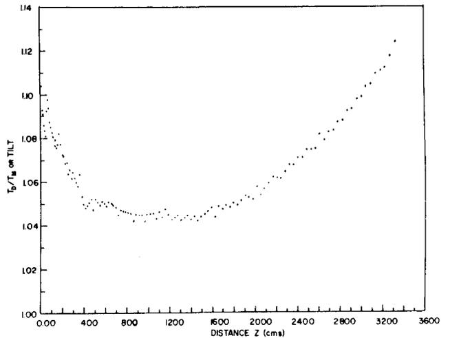
Fig. 10. Ratio of design transit time to measured transit time in the ANL 50 MeV linac.
