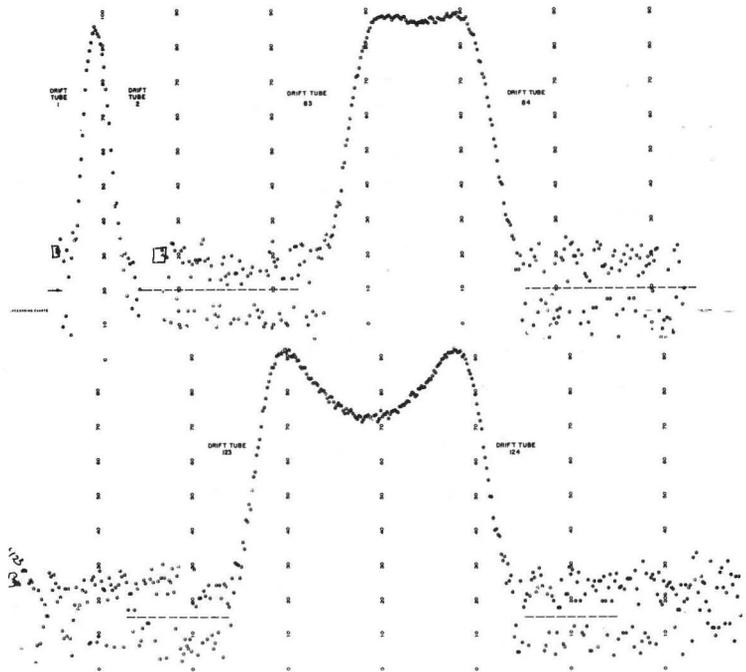
Fig. 2. A computer plot (shown at right) of actual measured fields at mm intervals along the axis for gaps 1, 83, and 123.
