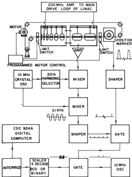
Fig. 1. Block diagram showing equipment used to digitally measure accelerating fields in the linac using perturbation techniques.
