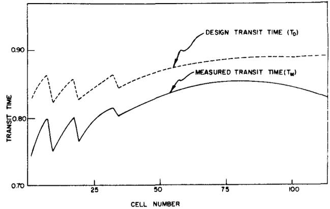
Fig. 9. Plot of design transit times and measured transit times in the ANL 50 MeV linac.
