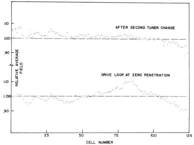
Fig. 3. Two typical plots of average accelerating fields for each cell along the linac.
