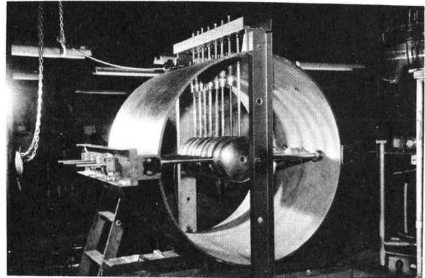
Fig. 4. Ten drift-tube test cavity.
