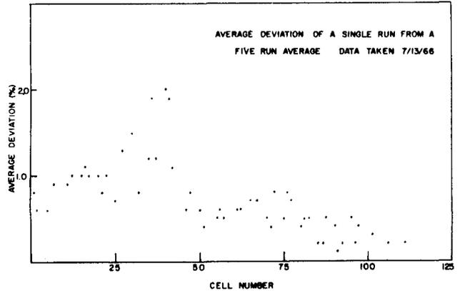
Fig. 8. Relative accuracy of measurements as determined by average deviation for values in single determination from 5-run average.
