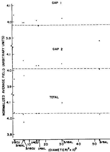
Fig. 6. Integrated fields normalized to unit ball volume vs ball (diameter)<sup>3</sup> to determine effect of ball size on measurements for gaps 1 and 2, and total of 9 gaps.
