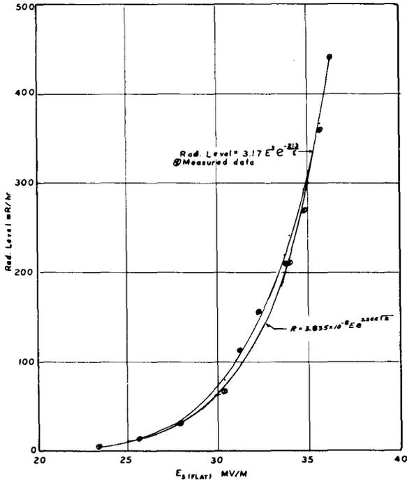
Fig. 5. Radiation level as a function of maximum field (5 MeV configuration).
