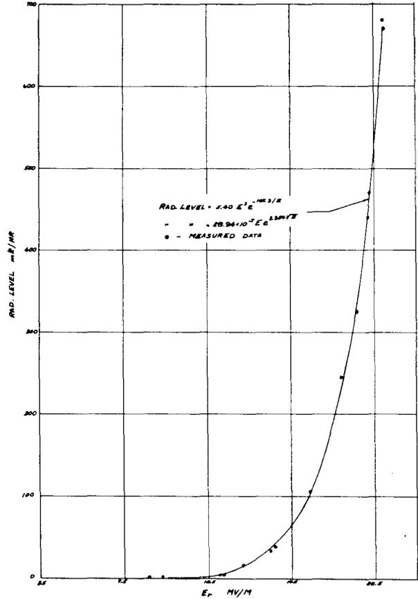
Fig. 6. Radiation level as a function of maximum field (50 MeV configuration).
