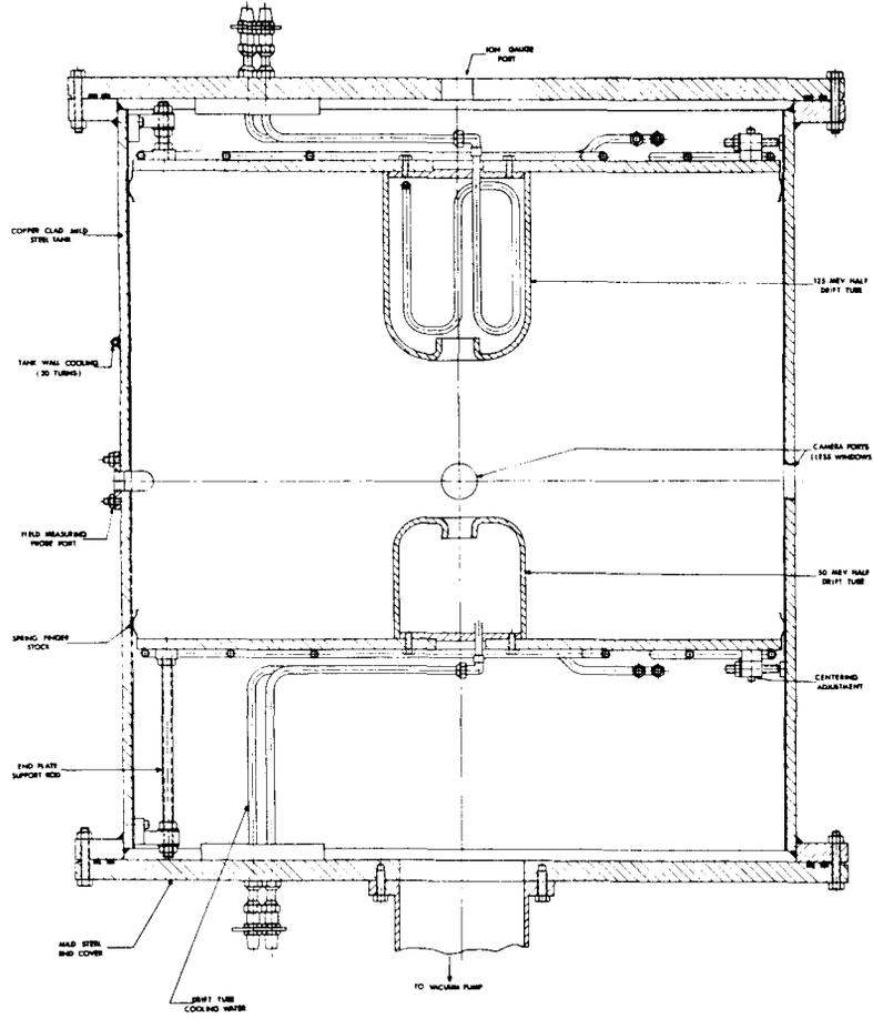
Fig. 2. Section view of sparking cavity with the 50 MeV drift tube (bottom) and the 125 MeV drift tube (top).
