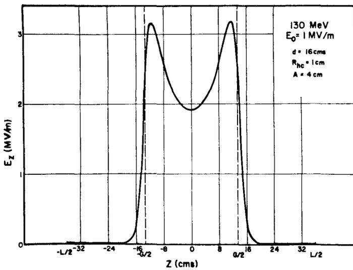
Fig. 3. Field distribution on the axis for 130 MeV geometry.
