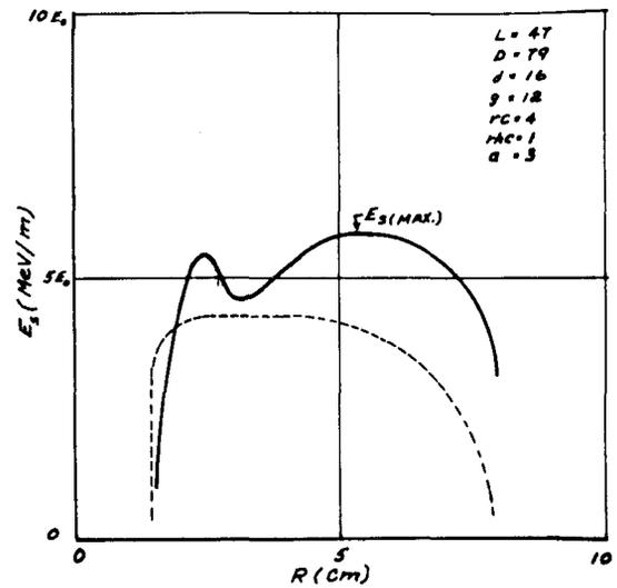
Fig. 4. Surface field of 50 MeV drift tubes.
