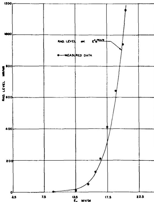
Fig. 7. Radiation level as a function of maximum field (130 MeV configuration).
