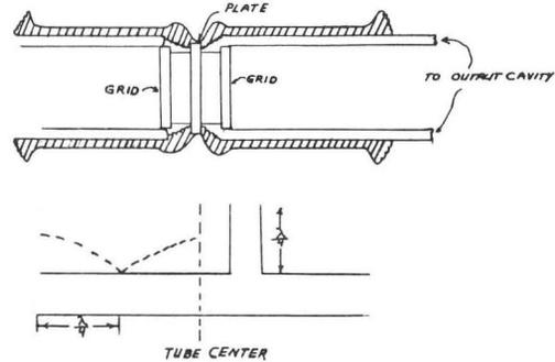
Fig. 3. Sketch of output cavity.
