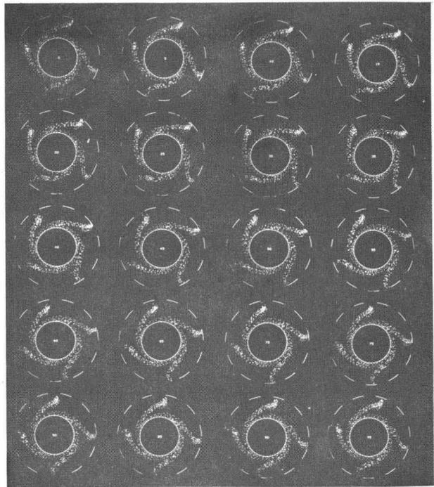
TIME SEQUENCE OF SPACE-CHARGE "SNAPSHOTS" IN THE QK630 AMPLITRON
