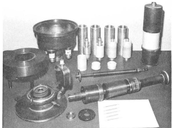
Fig. 11. Coaxitron parts.
