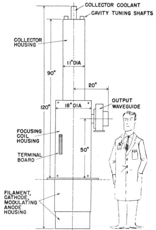
805 Mc, 1.25 Mw LINAC KLYSTRON
