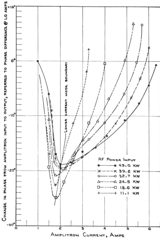
Fig. 7. Phase shift vs Amplitron current and drive.
