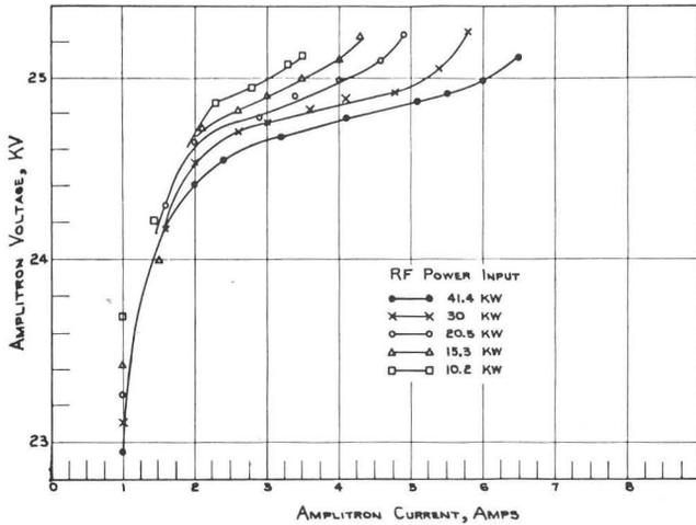
Fig. 5. Anode characteristics for QKS 1461.
