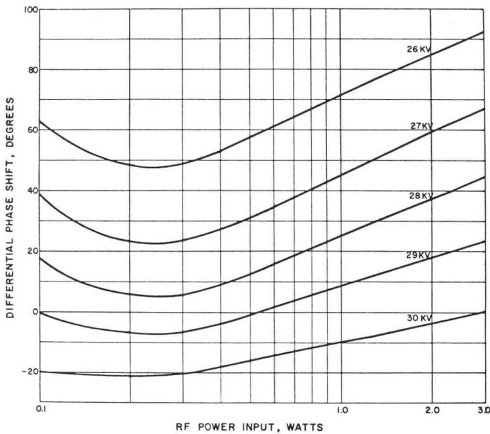
Fig. 18. Phase shift vs drive and beam voltage (Eimac).
