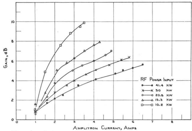
Fig. 6. Gain vs power input and current, QKS 1461.
