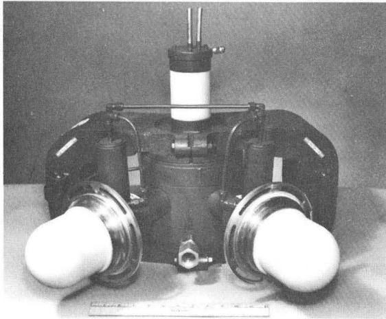
Fig. 3. 100-kW Amplitron, the QKS 1461.
