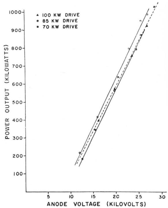
Fig. 15. Coaxitron output vs anode voltage and drive.
