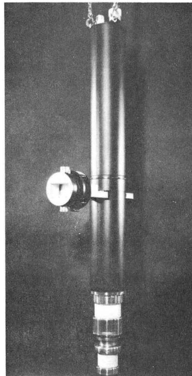
Fig. 20. Litton klystron, peak power 1.25 MW, duty 6%, frequency 1250 MHz.
