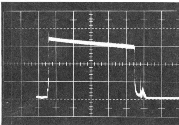
Fig. 8. Output pulse of Amplitron operating near the middle of its range; RF power input 22 kW; vertical scale, 1 A/cm; horizontal scale, 50 μsec/cm. Droop in pulse is a result of condenser bank droop.
