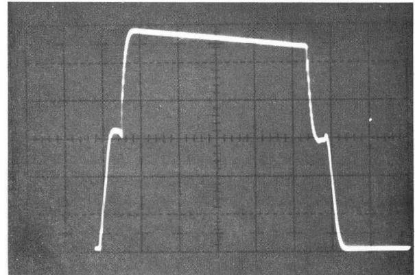
Fig. 10. Amplitude of rf field in 40-cell cloverleaf accelerator section (model B) with approximately 40-kW rf drive to Amplitron and Amplitron current near upper mode boundary. The klystron pulse overlaps the Amplitron pulse at beginning and end, and is fed through to output.
