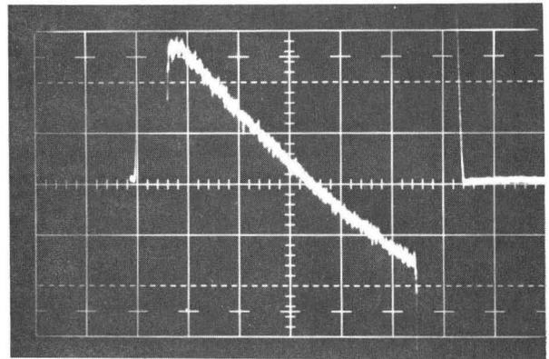
Fig. 9. Phase difference between rf waves into and out of Amplitron at current level and conditions of Fig. 8. Vertical scale 1°/cm, horizontal scale 50 μsec/cm. Change in phase shift is result of condenser bank droop.
