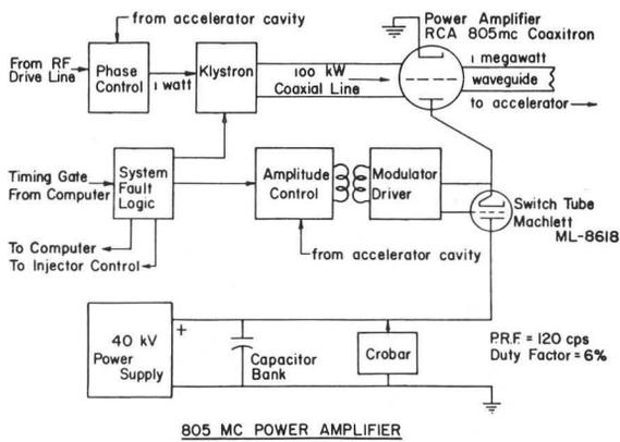
Fig. 14. Arrangement for coaxitron test.
