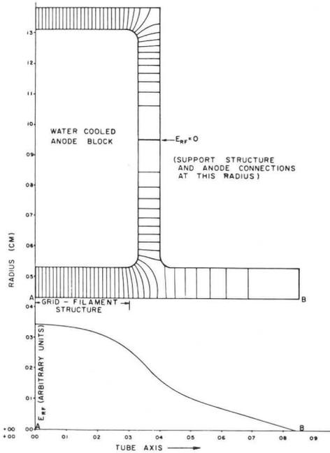
Fig. 13. Internal field plot of coaxitron.
