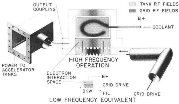
Fig. 12. Operating schematic of coaxitron.
