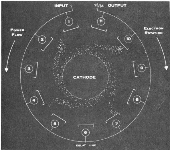
Fig. 1. Amplitron circuit, showing space charge.
