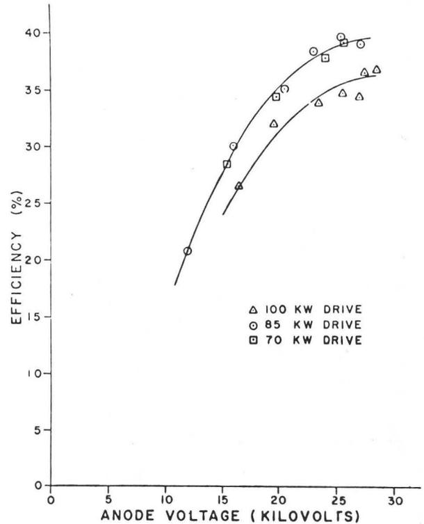
Fig. 16. Coaxitron efficiency vs anode voltage and drive.
