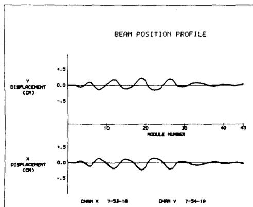
Fig. 5. Example of a graphical display which could be used to aid in steering the beam.
