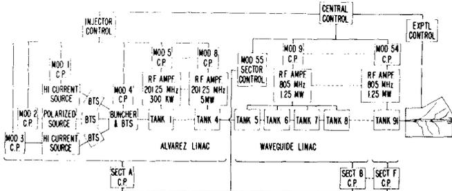
Fig. 1. Modular structure of LAMPF accelerator.
