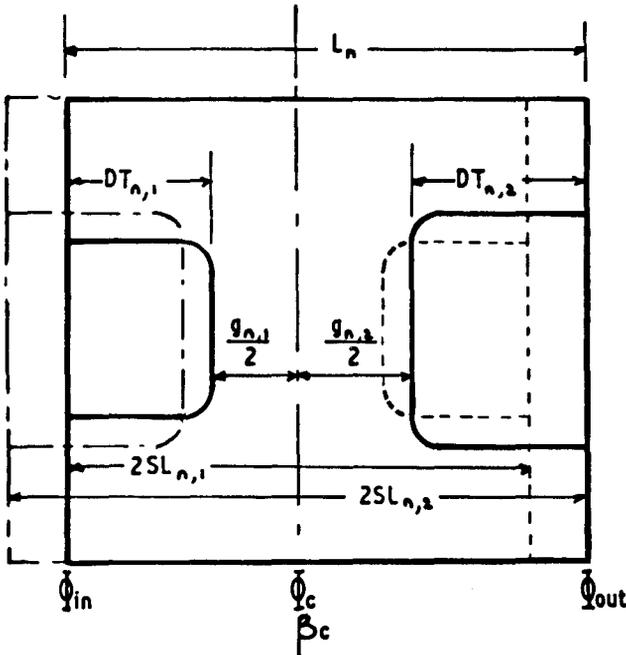
Fig. 2. General cell compounded from two symmetrical cells.
