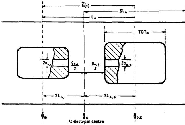
Fig. 1. General cell,  $n$ , of a linac.
