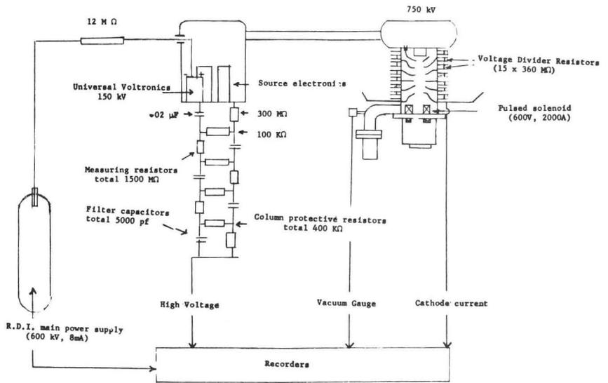
Fig. 7. Schematic of the test equipment.
