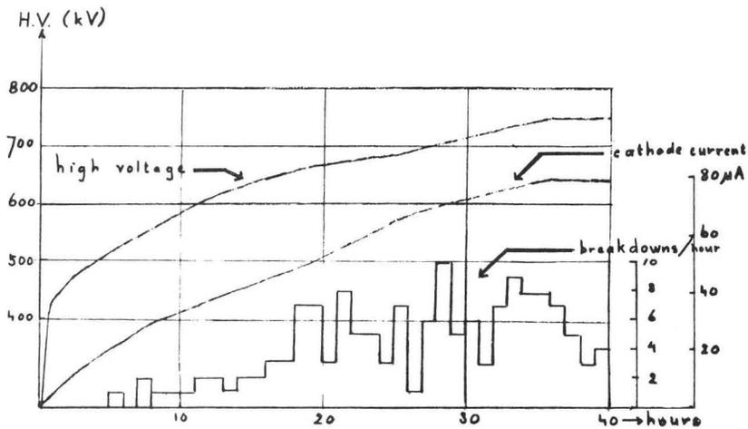
Fig. 8. A conditioning run of the high gradient tube.
