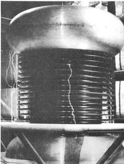
Fig. 6. The high gradient tube without humidity control.
