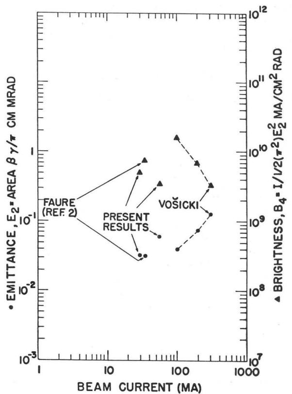
Fig. 13. Normalized emittance and brightness against beam current, measured at high energies (>100 keV).
