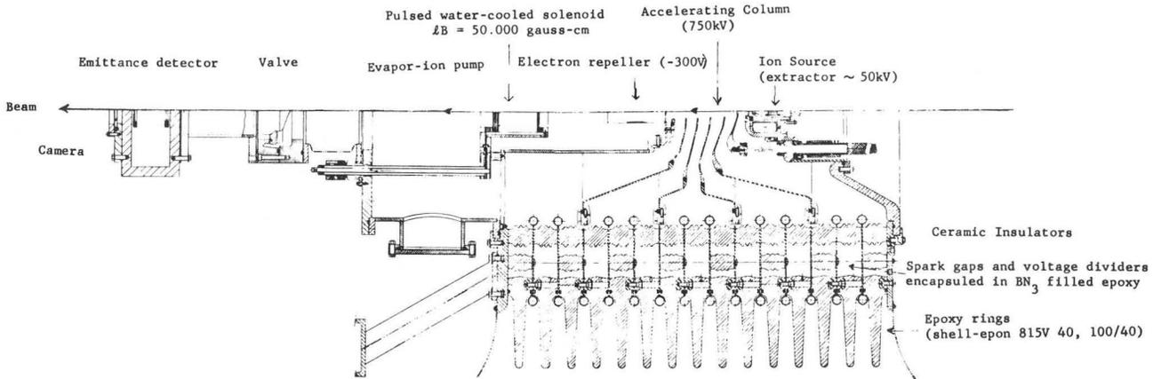
Fig. 5. The 750 kV high gradient pre-accelerator test setup.
