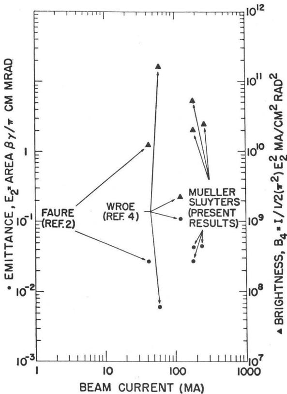
Fig. 12. Normalized emittance and brightness against beam current, measured at low energies (<100 keV).
