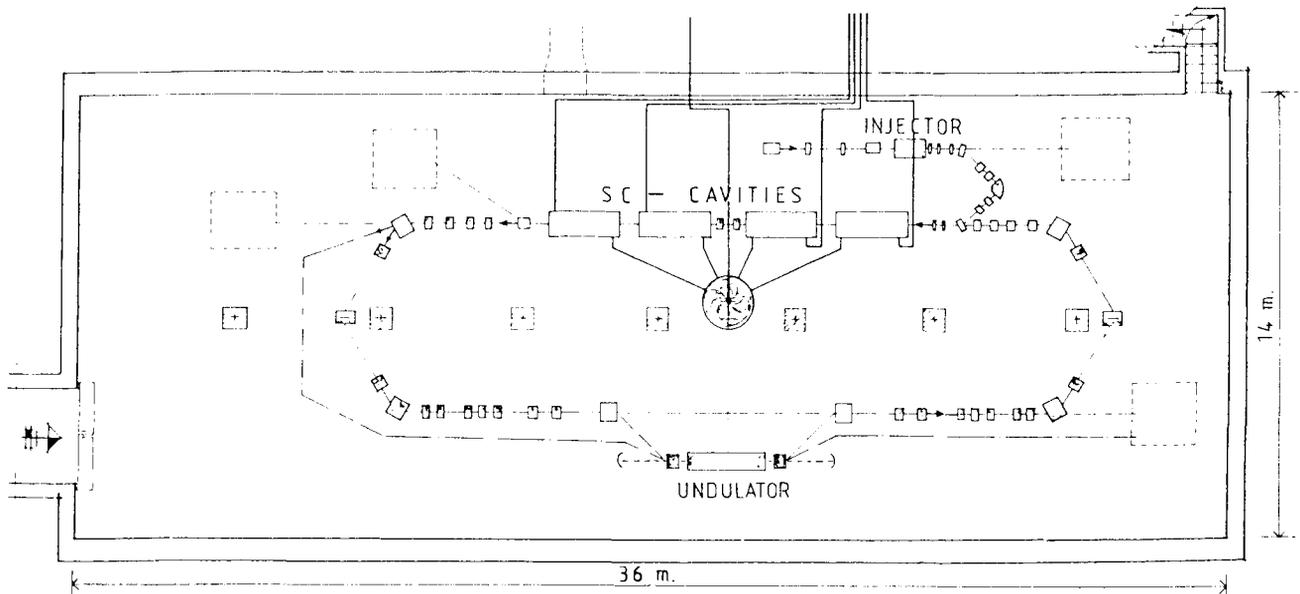
Fig. 1 - Schematic layout of LISA
