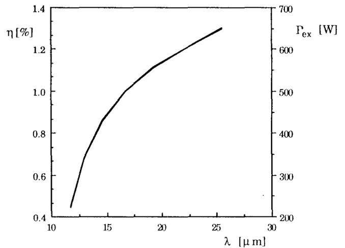
Fig. 4 - Average power and efficiency vs. wavelength during the macropulse.
