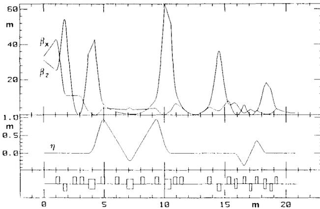
Fig. 3 - Optical functions in the transport channel in the isochronous configuration.
