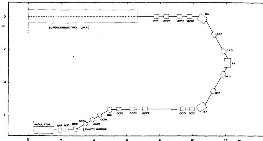
Fig. 2 - Layout of the SC Linac to the undulator transport channel
