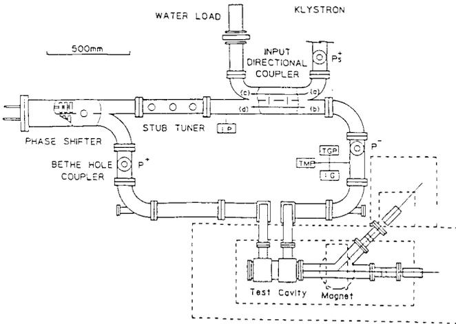
Fig. 3 Schematics diagram of resonant ring system.
