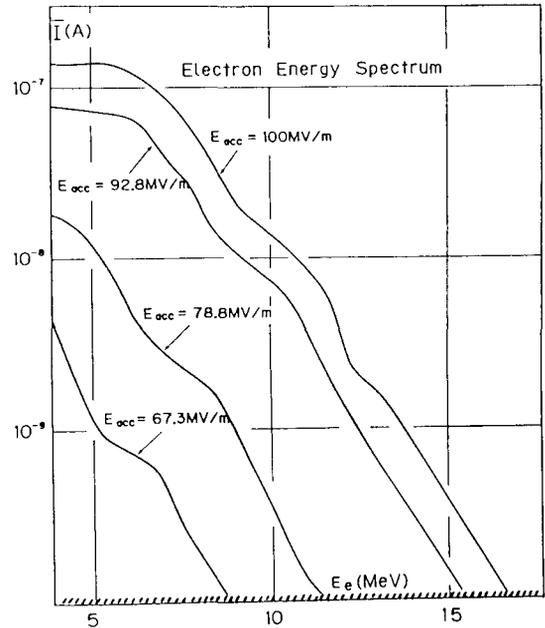
Fig. 4 Energy distribution of dark current electrons running out of the high gradient test structure.
