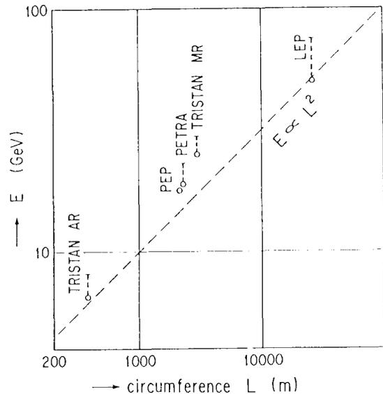
Fig. 1 Relation between beam energy E and ring circumference L of high energy electron rings.
