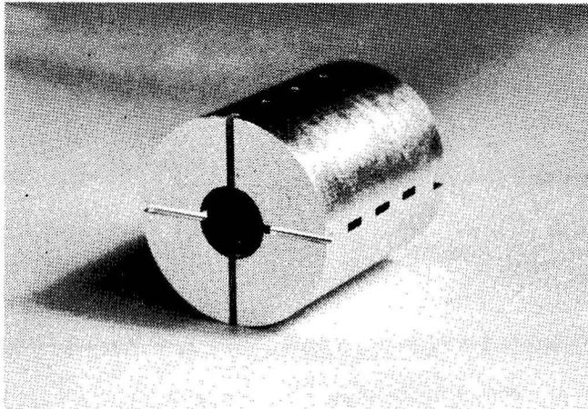
Fig. 3 Sample (one to one scale) of rectangular waveguide channels for damping and power feeders cut into copper by precision wire erosion.
