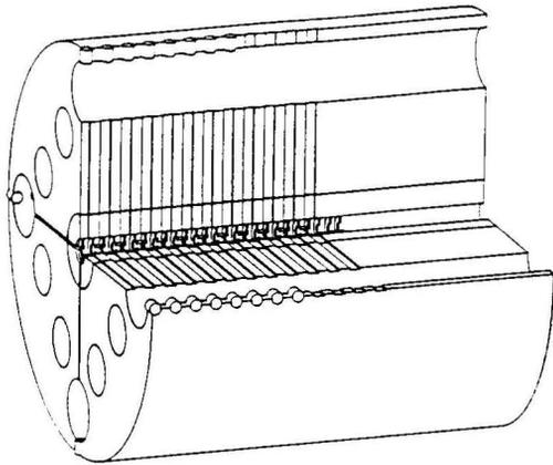
Fig. 2 Conceptual design of an accelerator unit containing the high-gradient structure (at the centre), damping and pumping slots, pump manifolds and cooling channels.
