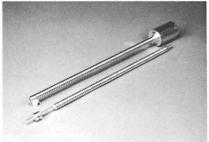
Fig. 1 Aluminium mandrels for electroforming of a complete 25 cm accelerating section. The piece in front includes cut-off pipes and a beam position monitor cell.
