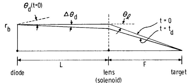
Fig. 3. Achromatic magnetic lens system consisting of a self-field lens (ion diode) plus a  $B_z$  solenoid lens.
