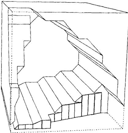
Fig. 10. Three-dimensional computer plot of the end region with a sloped undercut. The strips of surface area shown on the sloped cut and on the end of the overhang were used in computing the average power loss plotted below in Fig. 11.
