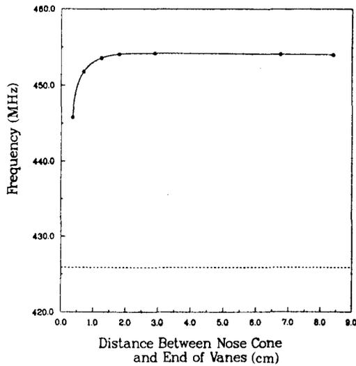
Fig. 4. Plot of the frequency of the end region with nose cone as a function of the distance between the nose cone and the end of the vanes. The curve is drawn to guide the eye, and the dotted line dictates the tuned frequency of the end region.
