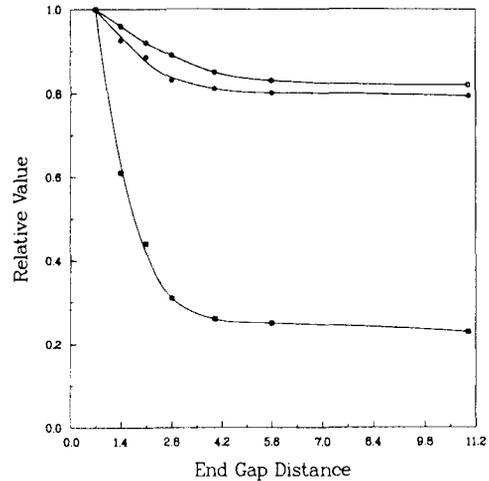
Fig. 7. Plots of the relative overhang length (top curve), the peak current density (middle curve), and the power loss caused by the end region (bottom curve) as a function of end gap distance. The curves are drawn to guide the eye.
