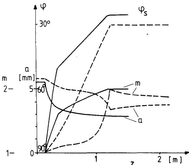
Fig. 3 The variation of the electrode parameters synchronous phase  $\varphi_s$ , modulation  $m$ , and aperture  $a$  along the  $z$ -axis. The dashed lines correspond to the standard method of RFQ design and the solid lines to the new method used in our design.
