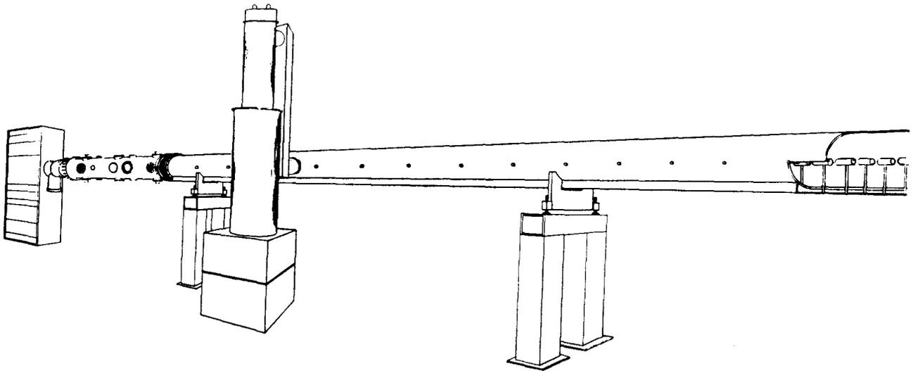
Figure 1: Artist's conception of a medical proton linac including source, LEBT, RFQ, drift tube linac, and power amplifier.
