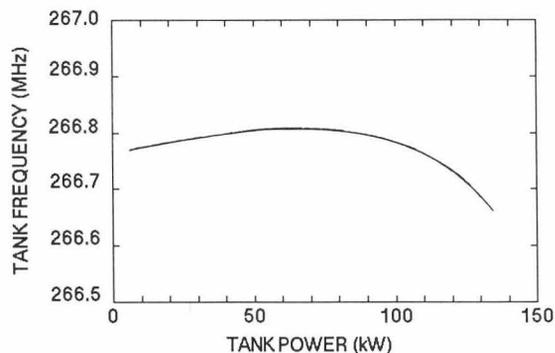
Figure 3: Frequency shift with tank power.
