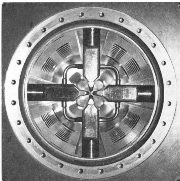
Figure 2: Axial view of RFQI cavity.
