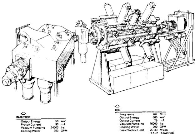
Figure 1: Accelerator components and layout.
