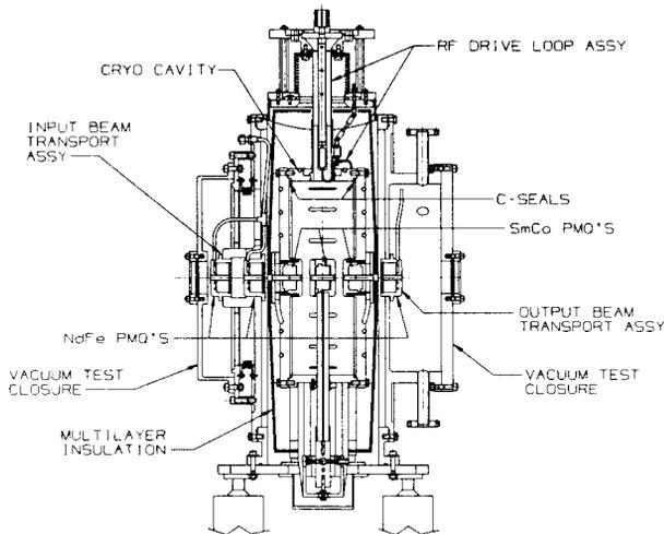
Fig. 2. Longitudinal cross section.
