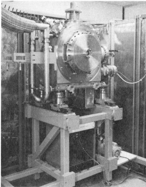
Fig. 3. CDTL in off-line test.
