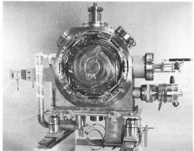
Fig. 4. CDTL Assemble - cryostat end closure removed.
